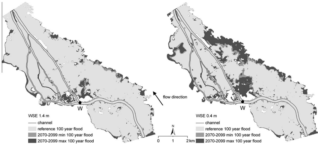
**Fig. 11.** Present and future inundation areas along Kokemäenjoki at the city of Pori. The 100-year flood simulations were performed for downstream boundary water surface elevations (WSE) of 1.4 and 0.4 m. W = location of water levels presented in Table 6.
