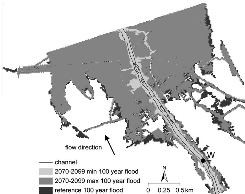
**Fig. 10.** Lapuanjoki north-west from the Lapua settlement center. The area consists mainly of fields and housing areas. Inundation area was reduced greatly in the minimum future scenario compared to the reference period. W = location of water levels showed in Table 6.
