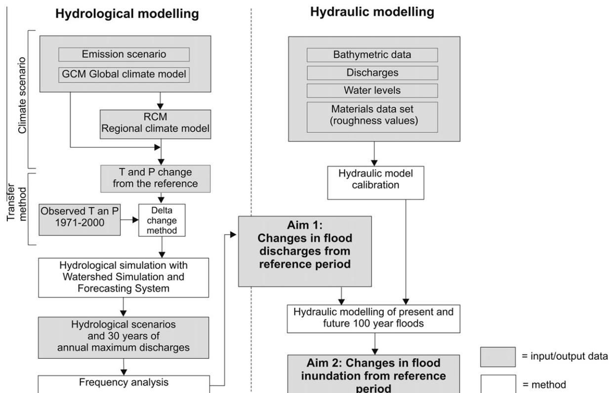
**Fig. 2.** Schematic representation of the method used in flood assessment. Climate scenario information is transferred to the hydrological model with the delta change approach and frequency analysis is performed on the simulated hydrological scenarios. The results of the hydrological modelling are used as input for flood inundation analysis.
