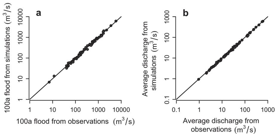
Fig. 4. Comparison of simulated (with observed temperatures and precipitations) and observed values in 1971–2000 at 67 sites: (a) 100-year floods with the Gumbel distribution and (b) average discharge.
