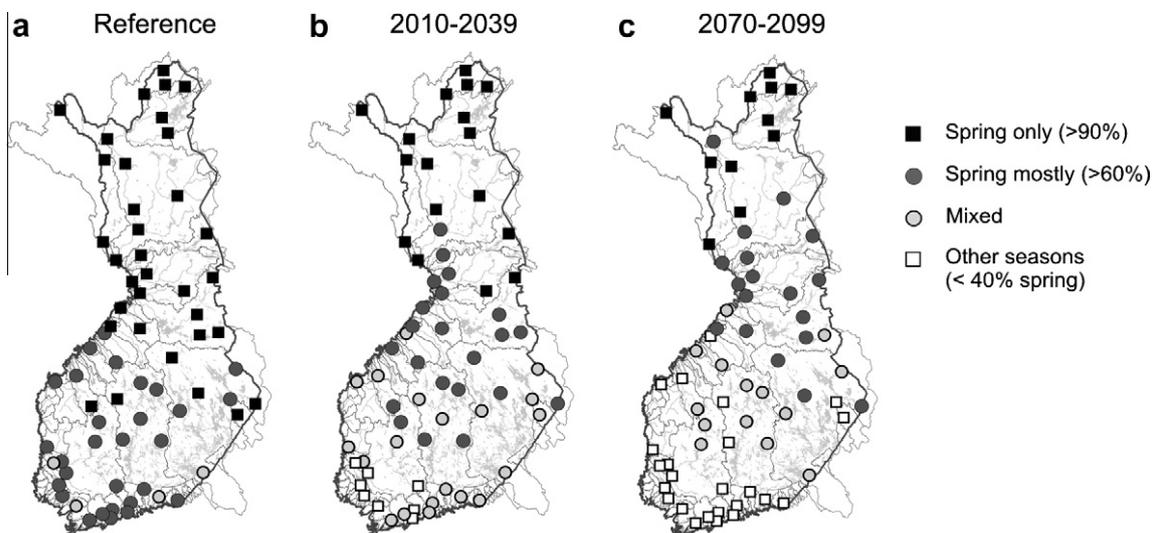
**Fig. 7.** Timing of the simulated annual maximum floods (% of spring floods, March–June) in the reference period (a, left), and in 2010–2039 (b, middle) and in 2070–2099 (c, right) with the median scenario.
