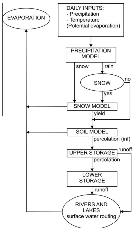
Fig. 3. The basic structure of the Finnish watershed model WSFS; see main text for further explanation (adapted from Vehviläinen et al., 2005).
