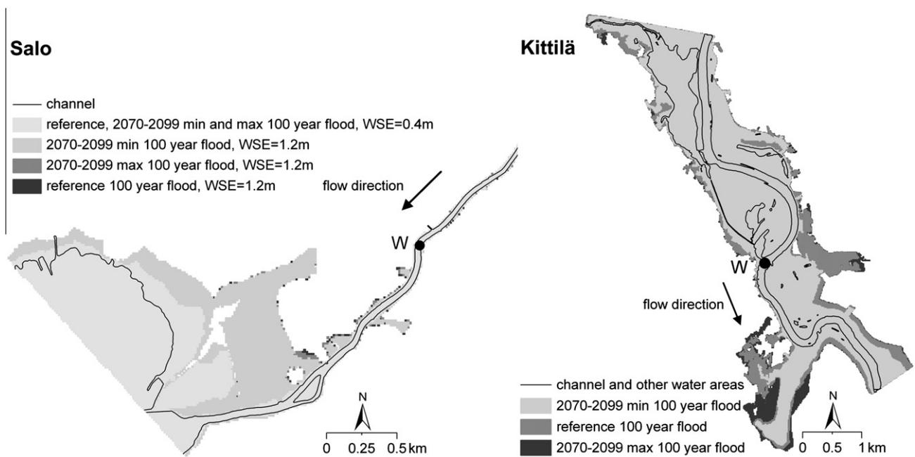
**Fig. 12.** The rivers Uskelanjoki at the city of Salo (left) and Ounasjoki at Kittilä municipality center (right). In Salo, simulations were performed for downstream boundary water surface elevations (WSE) 1.2 and 0.4 m. With 0.4 m WSE (lightest color), the inundation extents were almost equal with reference period, but also future minimum and maximum discharge scenarios. W = location of water levels shown in Table 5.
