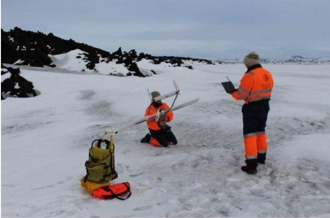
Recovery of fixed-wing drone, seconds after landing at the southeast edge of the lava by Jökulsá á Fjöllum. Photo: Morten S. Riishuus.
